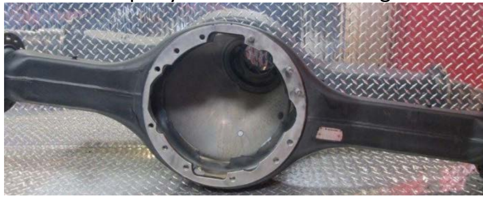
Properly cleaned axle housing
