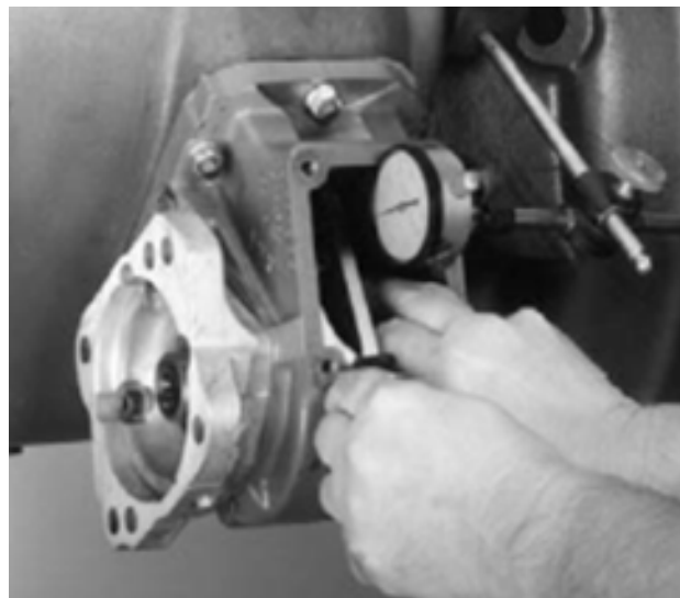
Backlash check using dial indicator
